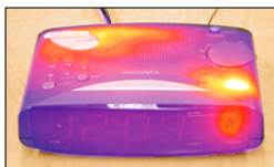
Multi-spectral imaging reveals a spycam hidden in the front right corner of a working clock radio.
